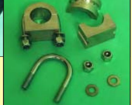
Solid Mounting Kit (alloy) (1) RR1370 Replaces original rubber mountings and clamps. Provides more positive feel to steering. Note: also transmits more road noise and vibration.
