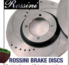
Rossini performance drilled and grooved discs are made from the best compounds with carbon & added manganese, molybdenum & titanium. The drillings cool the disc to reduce brake fade. The grooves reduce pad glazing and increase grip. The embedded Rossini logo on the disc face lets you know when they need replacing. Can be used with standard or 'Green Stuff' Kevlar Pads.
