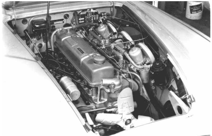
Rare factory publicity photo of tri-carb installation, marked "Confidential until Sept.20".
